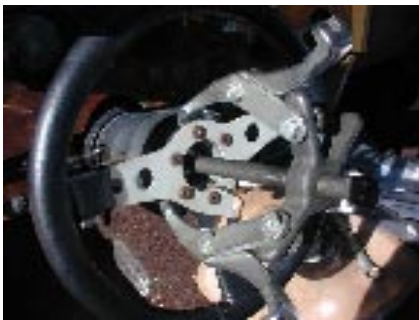
Using a puller to remove the hub adapter
