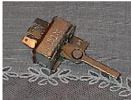
Heater Blower switch
